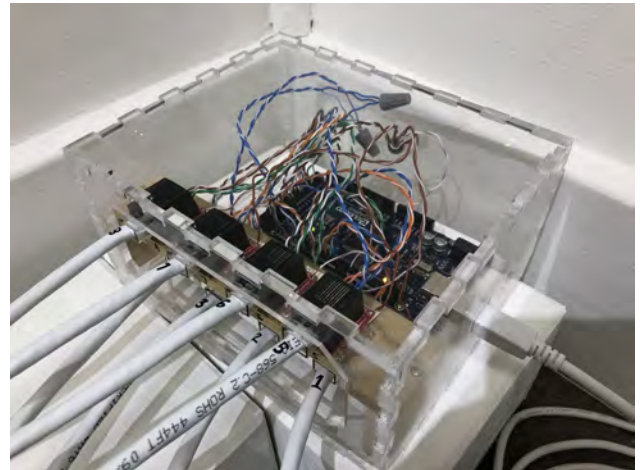
Figure 1: Wildfire motherboard (Arduino Mega2560) with eight Ethernet jacks for communication.
